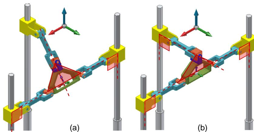
**Figure 4.** Two PRoM-120 configurations at the CKS or the combined transmission singularity: the first two links perpendicular to the first two prismatic joints and parallel to the platform plane while (a) the third links parallel to the platform plane and (b) the third limb perpendicular to the third prismatic joint.
