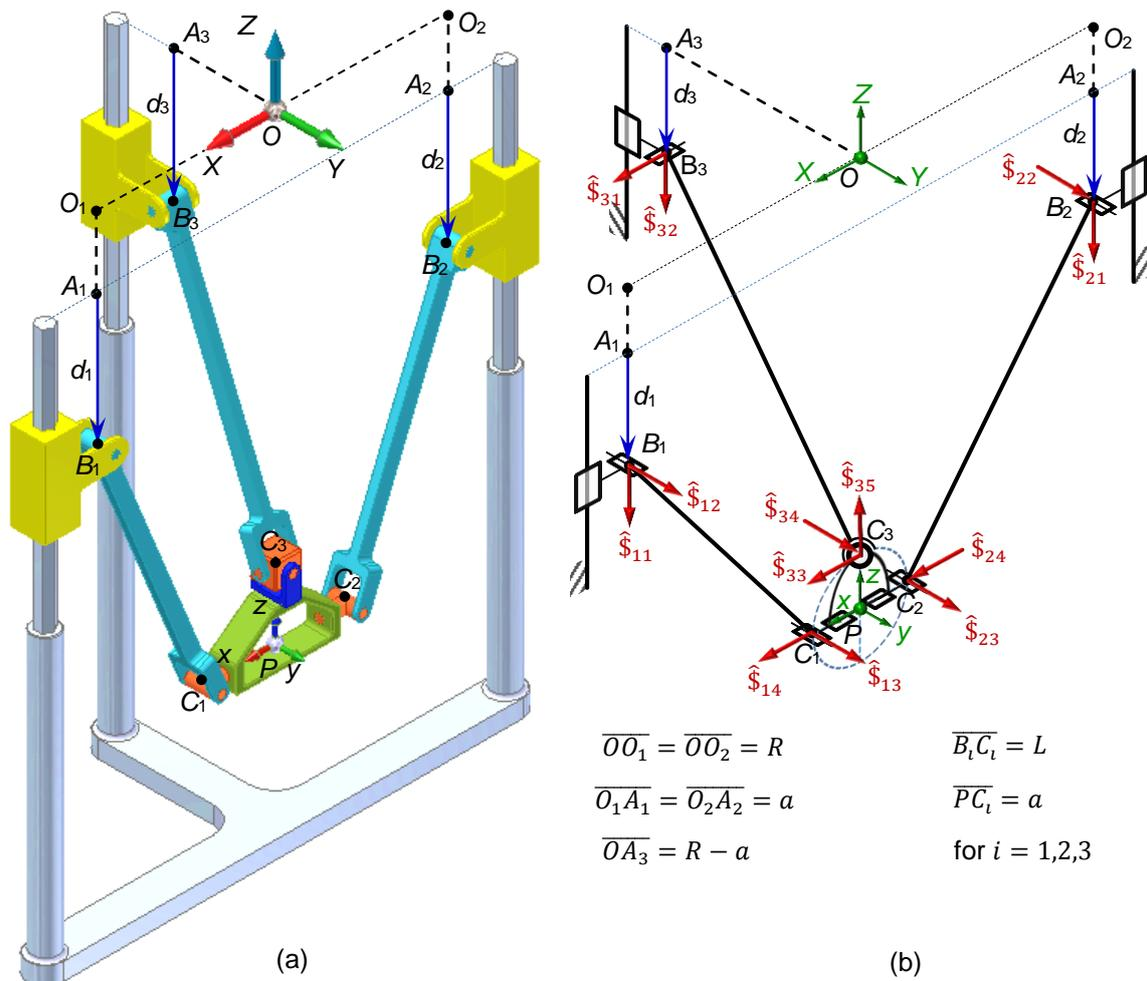
**Figure 1.** The geometrical architecture of PRoM-120 with 2-PRU/PRS kinematic chain: (a) simplified CAD model and (b) its kinematic diagram with the unit screw on each joint.
