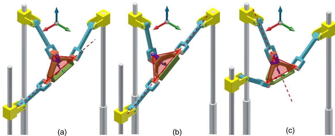
**Figure 3.** PRoM-120 configurations at the DKS or the output transmission singularity: (a) link  $B_1C_1$ , (b) both link  $B_1C_1$  and  $B_2C_2$ , and (c) link  $B_3C_3$  were in the plane to the platform plane, respectively.
