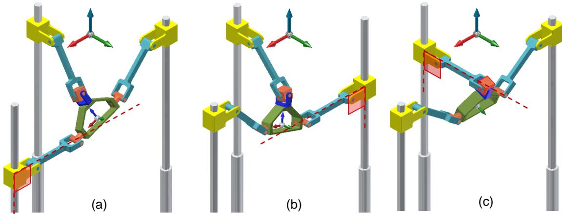
**Figure 2.** PRoM-120 configurations at the IKS or the input transmission singularity: (a) link  $B_1C_1$ , (b) link  $B_2C_2$ , and (c) link  $B_3C_3$  were perpendicular to the first, second, and third prismatic joint, respectively.
